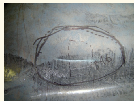
FIGURE [7] / Splits in original part geometry
