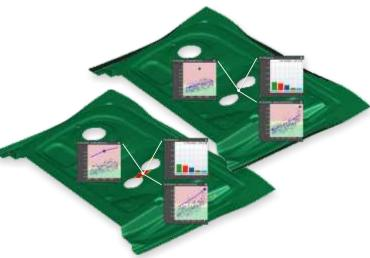
Design parameters which have the most influence on the stamped part can be identified during tool and process design
